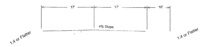
8" MDOT 21AA or 23A Limestone 8" MDOT Class II Granular Subbase
